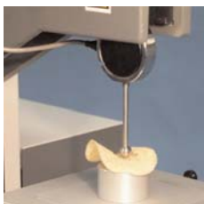
Crisp Fracture Test
